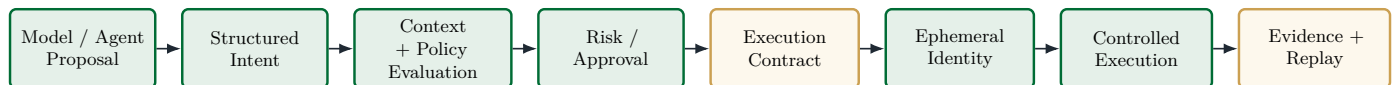
Figure 4.2: Agentic action lifecycle. ASCP converts an AI-generated proposal into governed execution through structured intent, policy evaluation, execution contracts, short-lived identity, controlled execution, and evidence capture.
